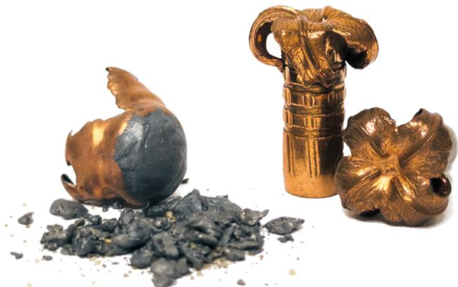
Left: A spent lead bullet with lead fragmentation debris. Right: A spent copper bullet with no fragmentation.
